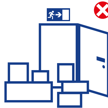
Escape routes - wrong
